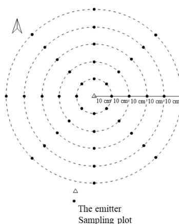
**Figure 2.** Distribution of soil salt crust (SSC) sampling plots around the drip irrigation emitter.
