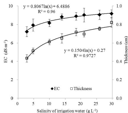
**Figure 4.** Variations in EC and thickness of soil salt crust drip irrigated with waters of different salinity levels in the Taklimakan Desert Highway Shelterbelt (corresponding sampling locations were shown in Figure 1). Error bars show 1 standard deviation.
